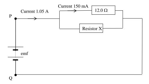
a) Calculate the value of Resistor X to ensure that a current of 150 mA flows in the 12.0  $\Omega$  resistor when a current of 1.05 A flows from the source of emf.
